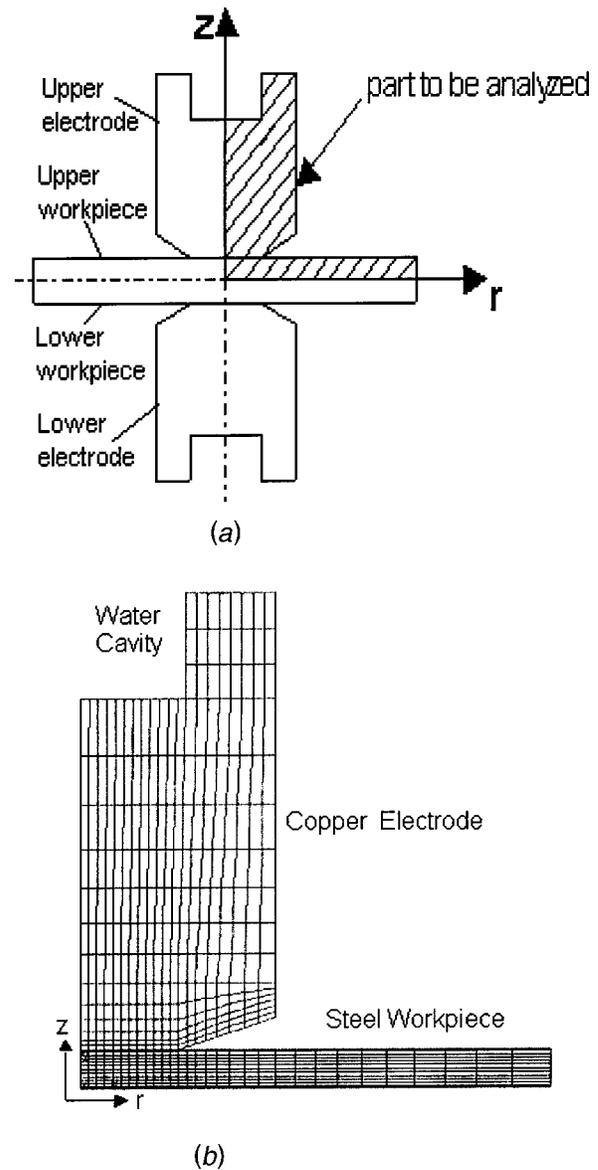
Fig. 1 (a) Axisymmetric mode of spot welding setup (b) Finite element model for spot welding
