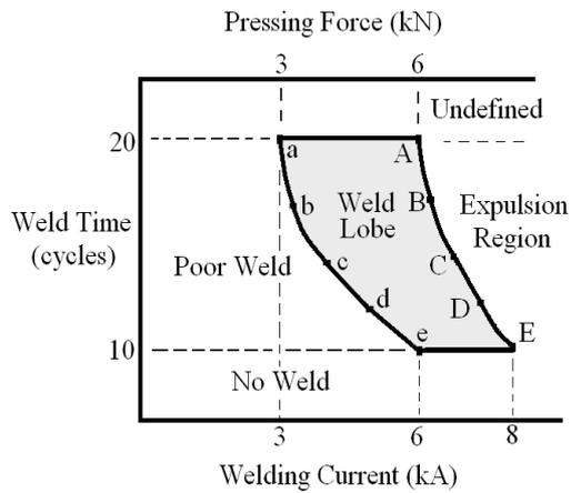
Figure 2 Weld Lobe for 1mm Sample Sheets.
