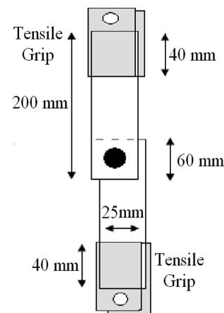
Figure 1 Test Sample
