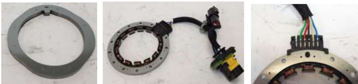
Fig 1: VR resolver used in Edrive system
