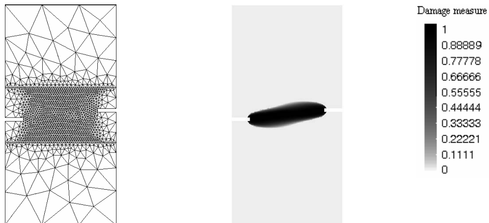
Figure 7.3: Crack pattern obtained with very fine FE mesh
